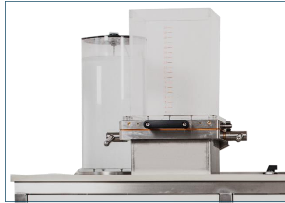
Former column & white water system
